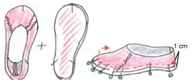
Insert the pins perpendicular to the sewing direction.
