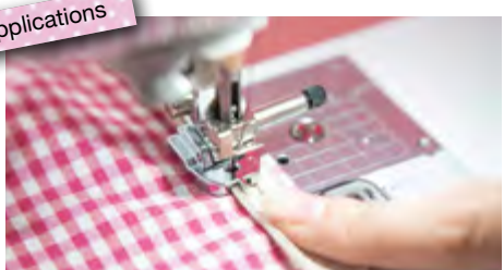
Specialized presser foot can be guided over a concealed zipper - easy enough for anyone to sew neat finishes.
